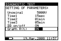
Fig. 19. Set-up menu in Diagnostic Test measurement
