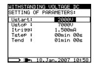
Fig. 29. Set-up menu in Withstanding Voltage function
