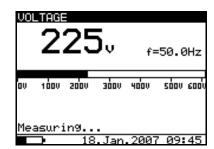
Fig. 9. Voltage function display states
