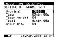
Fig.12. Set-up menu in Insulation Resistance measurement
