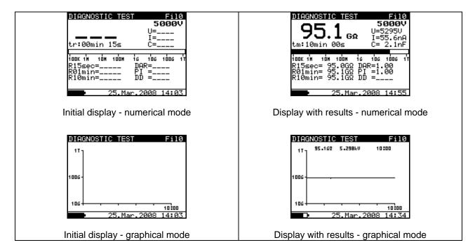
Fig. 16. Diagnostic test display states - Graph R(t) enabled
