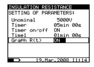
Fig. 13. Set-up menu in Insulation Resistance measurement
