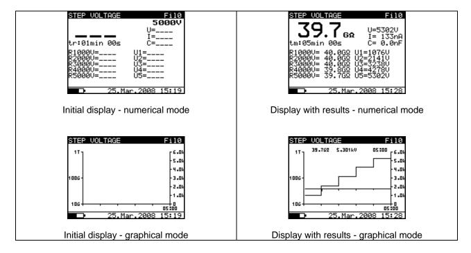
Fig. 22. Step Voltage function display states - Graph R(t) enabled
