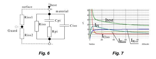
R<sub>iss1</sub> and R<sub>iss2</sub> - the surface resistivity (position of optional guard connection)
