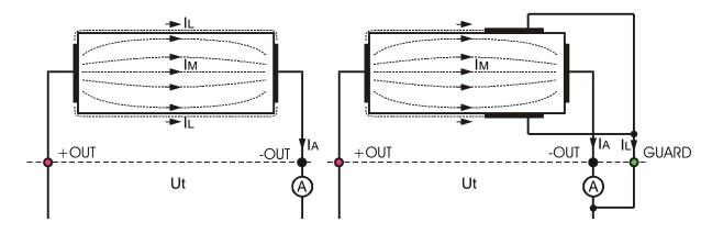
Fig. 8. Connection of GUARD terminal to measured object
