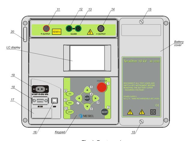
Fig. 1. Front panel
