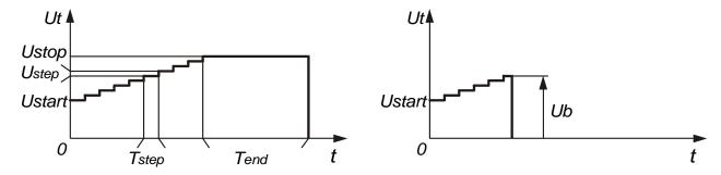
**Fig. 27.** Test voltage presentation without breakdown (left part) and with breakdown (right part)
