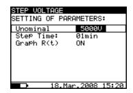
Fig. 24. Set-up menu in Step Voltage Test
